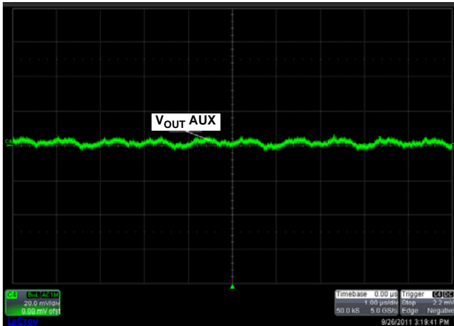
FIGURE 7. ISL70001SRH AUXILIARY VOLTAGE RIPPLE
